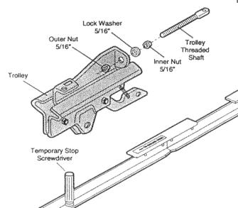
As a temporary stop, insert a screwdriver into the hole in the front end of the T-rail.
